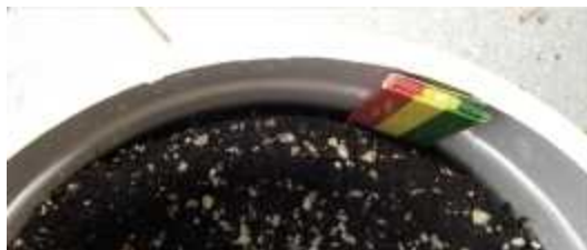
Soil shrinks when dry; it causes a gap to form alongside the container wall.
