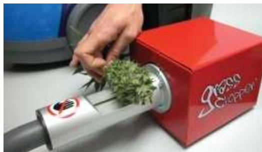
The Grass Chopper is one of the many new medium-sized bud trimmers that feature vacuum leaf removal.
