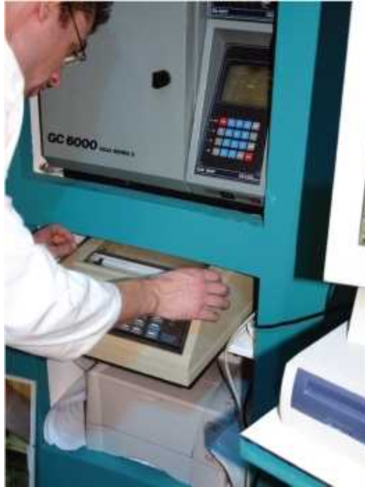
This scientist from Canna measures the exact THC content of harvested buds with a gas chromatograph.
