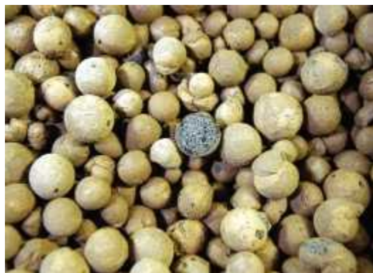
Expanded clay holds moisture and nutrients along with lots of oxygen.
