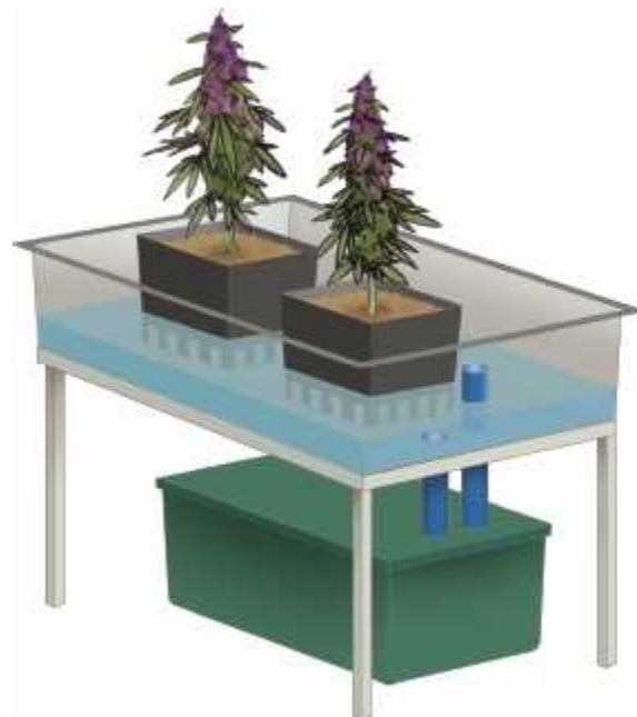
Nutrient solution floods the growing bed and drains back into a reservoir in an ebb and flow garden.
