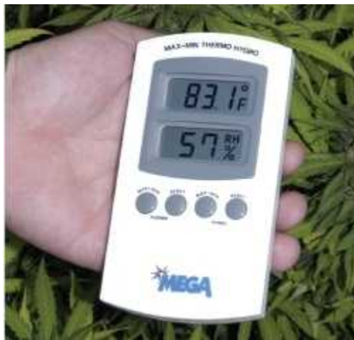
A maximum/minimum digital hygrometer registers the high and low humidity as well as current humidity.
